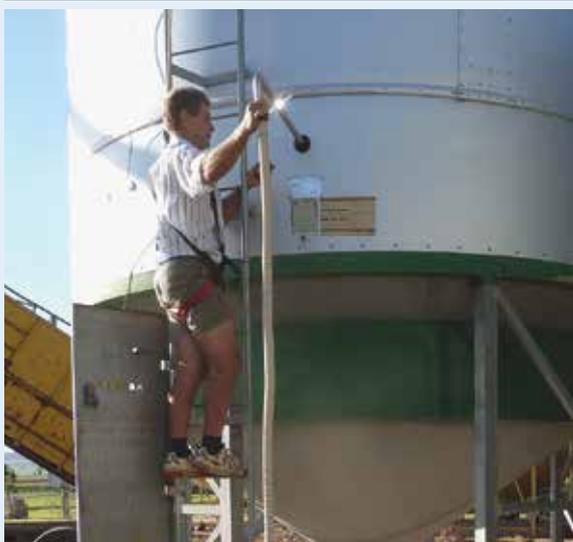
**Sample site:** Poly water fittings (40-50mm) mounted in the silo wall beside the ladder allow grain samples to be taken with a vacuum probe. Mounting them every few metres up the silo enables easy monitoring of the aeration drying front as it progressively dries grain from the bottom of the silo to the top.
